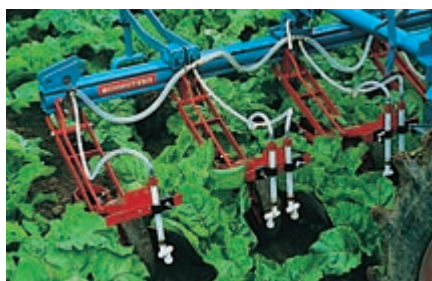
Underleaf spraying in row crops
