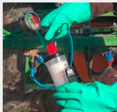
Calibrating twin flat spray nozzles with SPOTON
